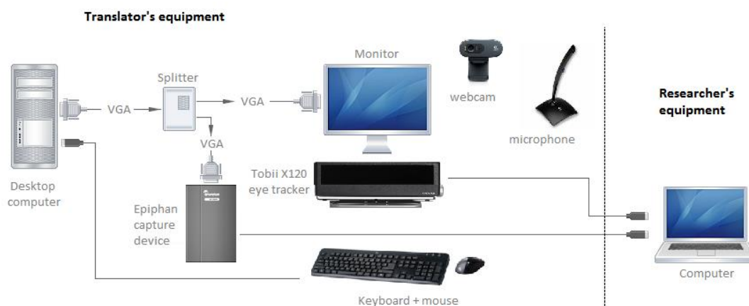
Figure 6. Simplified representation of the experimental set-up
