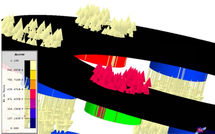
Fig 35. Demagnetized magnet in green, FEM model.
