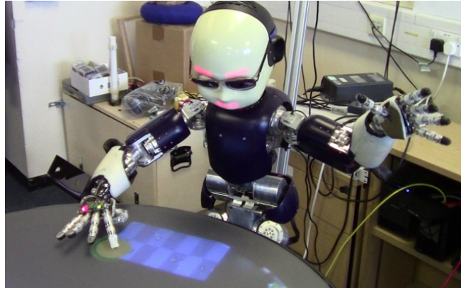
Figure 7.1: iCub interacting with the virtual keyboard shown by the Reactable tactile interface. The finger is used to control the virtual object, which is used by our software to know which sound to play.
