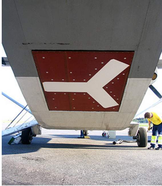
Fig. 3.4 AMIRAS installed on the HUT Skyvan. It is tilted about 24^\circ away from nadir in a similar configuration to that of SMOS [ESA SMOS website].
