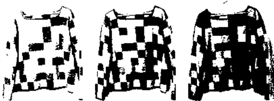
Figure 2.6: An image binarized at different threshold levels: a) 51 b) 77 and c) 102. The MSER regions are those that do not change (no pixel of its boundaries switches color) during several successive threshold levels.
