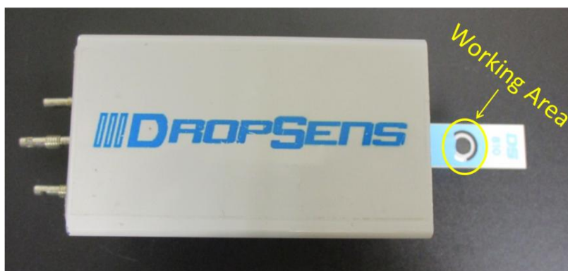
Figure 5.4. Bi-C SPE connector to the potentiostat
