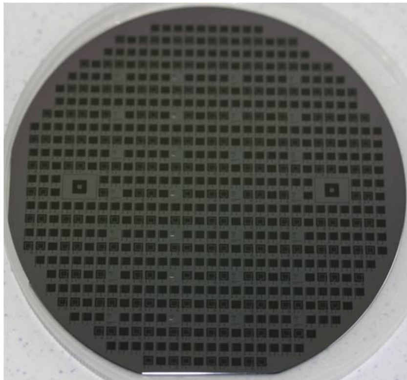
Figure 7.2. Image of a 4-inch wafer containing C/SiO 2 thin-film electrodes patterned by the standard photolithography process
