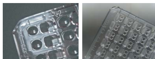
Figure 29: Details of MRC ™ Maxi Plates used for condition optimisation (left, 48-well plates) and screening (right, 96-well plate).
