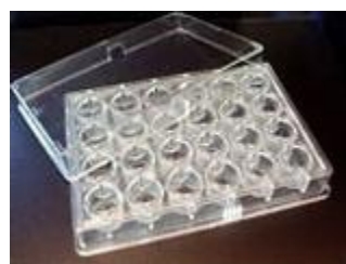
Figure 27: 24-well nongreased Linbro™ plates (Jena Bioscience, DE) used for hanging drop crystallisation.
