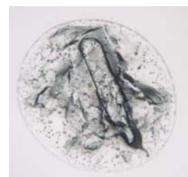
Figure 63: Salt crystals formed from an RNase7-A75H88 sample at 20 mg/mL and 20 ^\circ\text{C} . Sitting drop and reservoir volumes are, respectively, 0.2 and 50 \mu L. Crystallisation condition is 1.26 M (\text{NH}_4)_2\text{SO}_4 , 0.1 M CHES-NaOH pH 9.5 and 0.2 M NaCl, using 5 mM 3'-CMP as cocrystallant.
