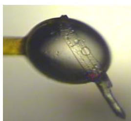
Figure 58: ECP crystal obtained by the hanging drop methodology. Total volumes of drop and reservoir were, respectively, 0.2 and 45 \mu\text{L} . The mixture is composed of 0.2 M \text{Li}_2\text{SO}_4 , 0.1 M TRIS-HCl pH 8.5 and 15% PEG4000. Protein concentration is 14 mg/mL. Incubation temperature was 20 ^\circ\text{C} .
