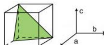
Figure 34: Plane with Miller indices (hkl) (211) in a cubic crystal depicted in green. Intersection points are a/2 , b/1 and c/1 .
