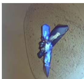
Figure 59: ECP crystal obtained in a hanging drop. Total volumes of drop and reservoir were, respectively, 2 and 800 \mu\text{L} . The mixture is composed of 0.2 M \text{Li}_2\text{SO}_4 , 0.1 M TRIS-HCl 0.1 M pH 8.5 and 15% PEG4000. Protein concentration is 14 mg/mL. Incubation temperature was 16 ^\circ\text{C} .
