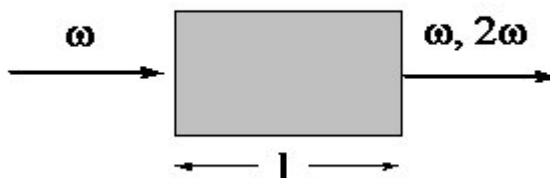
Figure 75. Generation of the second harmonic in a material of length l .
