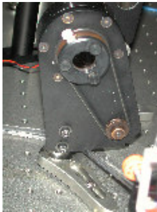
Figure 68. (a) Picture of the the set-up used for the picosecond transient absorption experiments in the laboratory of Prof. A. M. Brouwer at the University of Amsterdam, (b) Cell holder with fast rotation.
