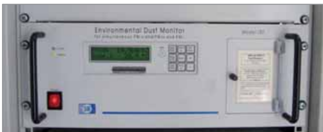
Figure 2.10. GRIMM monitor (model 180).
