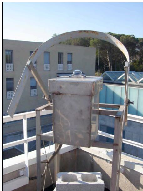
Figure 3.15: The Whole Sky Camera system from the University of Girona. The band shadows the camera in order to protect the CCD sensor.
