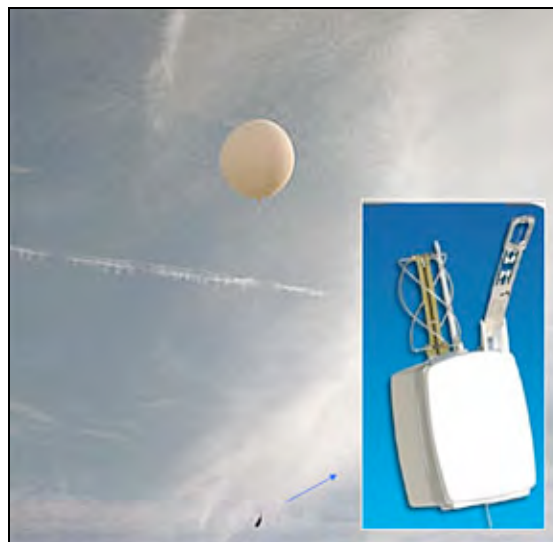
Figure 3.10: Vaisala RS92, an example of Radiosounding system, and the balloon for the launching. [Vaisala™]
