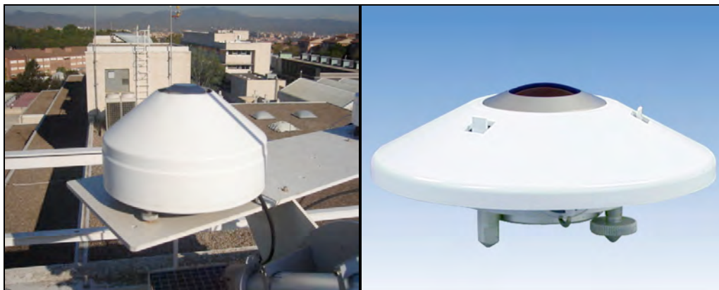
Figure 3.4: Pyrometers Kipp-Zonen CG1 at Girona (left) with ventilation and shadowing device, and Kipp-Zonen CG4 (right). The CG1 pyrometer has a flat silicon window, whereas CG4 has a meniscus window.
