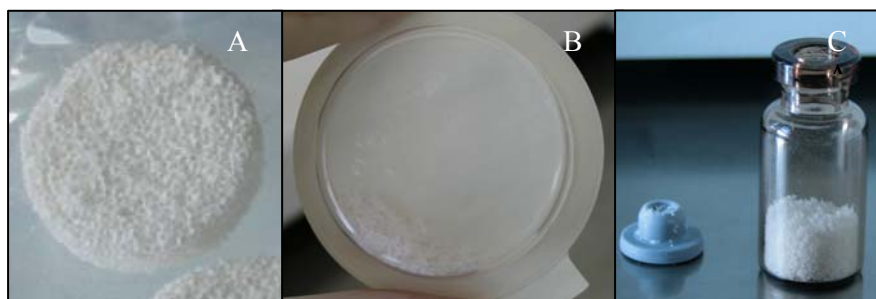
Fig. 14: Different types of calcium phosphate. A) Discs of pure HA showing the porosity of the material. B) Ceros ® TCP large particles used in this study. C) Biphasic calcium phosphate containing 20% HA and 80% \beta -TCP used in this study. HA, hydroxyapatite; \beta -TCP, \beta -tricalcium phosphate.
