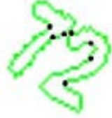
Figure 3.6: Initial segmentation points (black dot) found from concave residua after using polygonal approximation are shown on a touching component.
