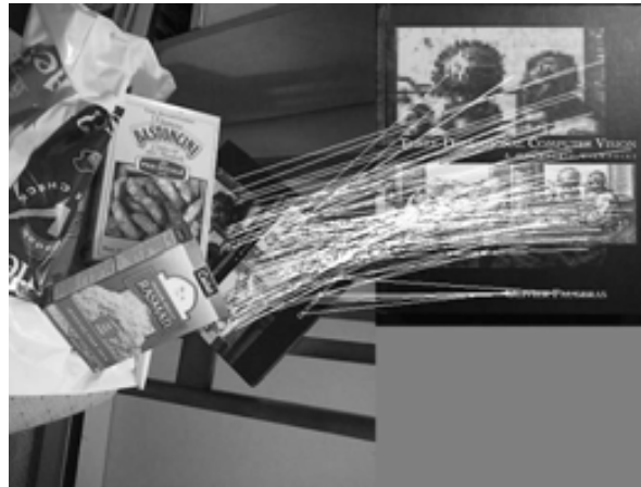
Figure 4.10: Example of object recognition with SIFT.
