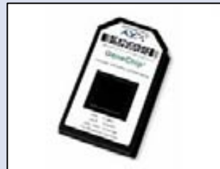
FIGURE 14 | Affymetrix GeneChip® microarray. Probes are located in the central glass surface enclosed within a sealed cartridge.
