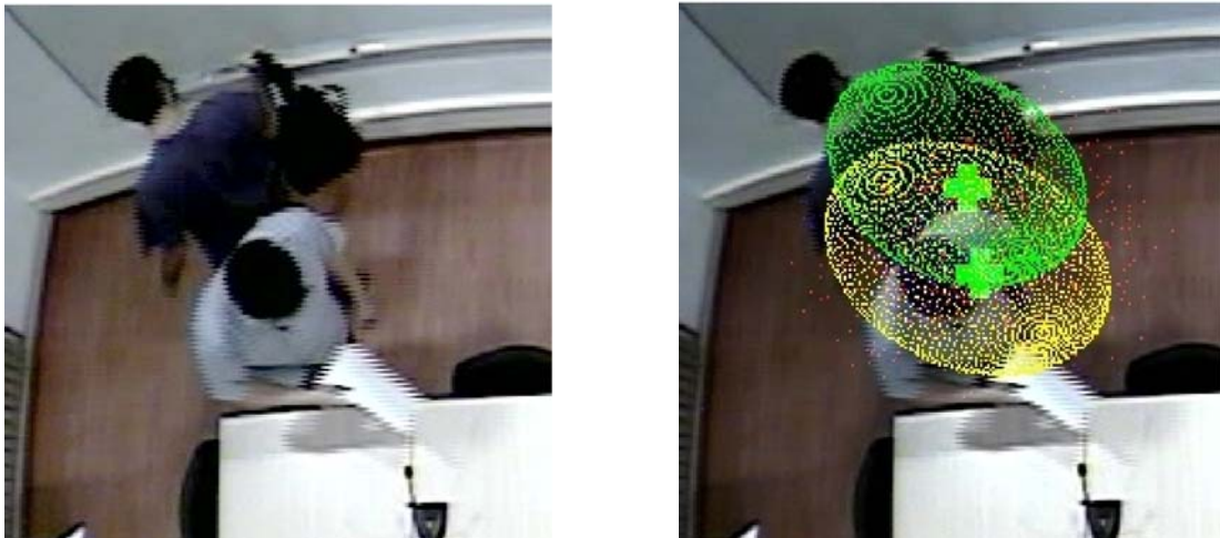
Figure 3.4.1. Particles from the tracker A (yellow ellipsoid) falling into the exclusion zone of tracker B (green ellipsoid) will be penalized
