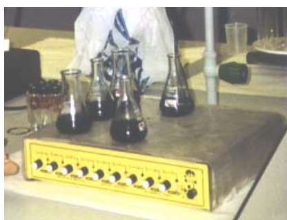
Figure 6.5. Isotherm adsorption batch tests.
