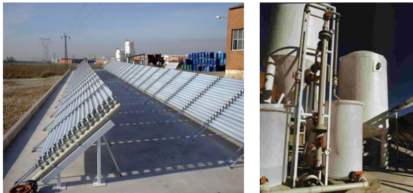
Figure 3.4. Images of the photoreactor (left) and the TiO 2 recovery system (right) of Hidrocen solar detoxification plant.
