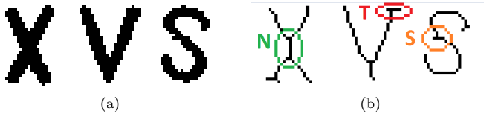
Figure 4.1: Usual thinning artifacts. (a) Original patterns. (b) Thinning results with artifacts (Necking: green, Tailing: red, Spurs: orange).
