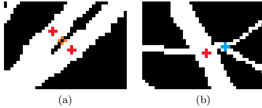
Figure 4.9: Error samples. (a) Caused by connectivity (orange: pixels causing connectivity). (b) Caused by proximity (blue: missing intersection).
