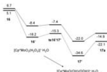
Figure 9: Energy profile (in kcal mol -1 ) for the activation of H 2 O 2 by [Cp*MoO 2 (H 2 O)] + in the presence of an additional H 2 O molecule in the gas phase (dashed lines) and in water solution (plain lines).
