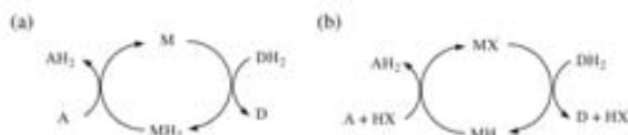
Scheme 3. (a) Dihydric route and (b) monohydric route. Metal complex (M), donor group ( DH_2 ), acceptor group (A), proton donor (HX).
