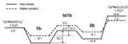
Figure 8. Relative energy profiles (in kcal mol -1 ) in the gas phase and a water solution for the starting complex ( 1b ), transition state ( ts1b ), and product ( 2b ) of eq 6.
