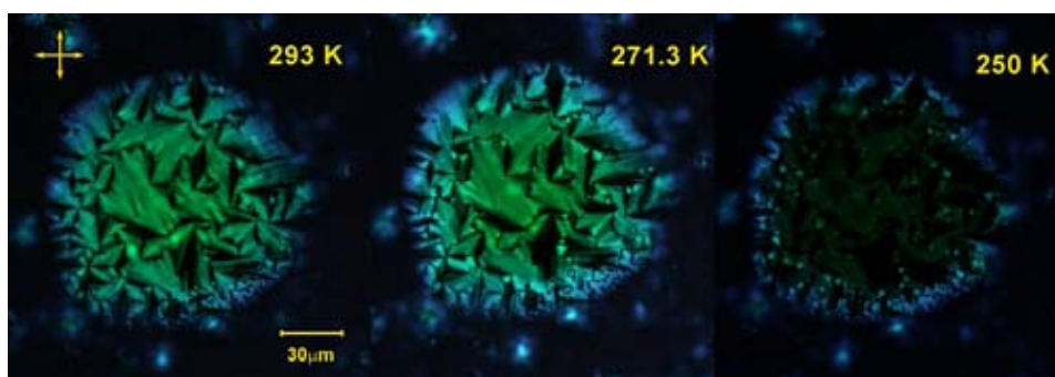
Changes in the optical texture while cooling down from 313 K using the cooling procedure described in section 7.
