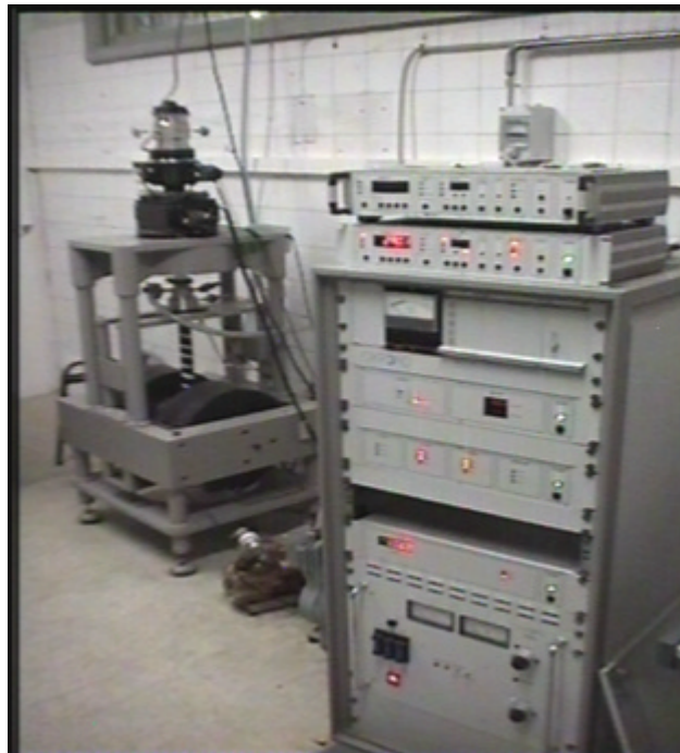
Figure 2.5: Photograph of the vibrating sample magnetometer used in the present study
