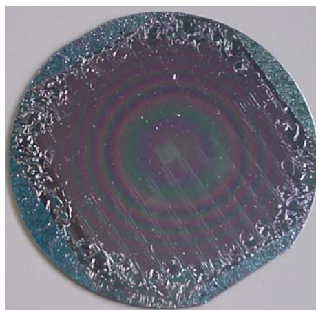
Fig 3.18: Effects of the excessive mechanical stress over silicon-based multilayer structures.
