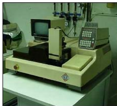
Fig 3.33 Diamond saw cutting technique and equipment used. It causes roughness at the optical device cross section that needs polishing.
