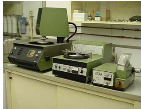
Fig 3.34 Polishing technique and equipment used so as to eliminate roughness from the optical waveguide cross section.
