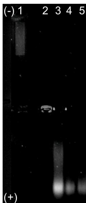
Fig. A2. Electrophoresis of UCNP before and after functionalization. Lanes correspond to samples (1) UCNP-APTMS, (2) UCNP-APTMS-BSA, (3) UCNP-APTMS-Dex, (4) UCNP-APTMS-BSA/Dex, and (5) UCNP-APTMS-BSA/Dex-Strv5.0. UCNP were revealed under 405 nm excitation wavelength.
