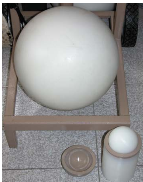
Figure 3.3: The 12" sphere with the 1 cm lead insert. The lead shield, formed by two half shells, is placed around an inner 3" polyethylene sphere which is held by a polyethylene cylinder.
