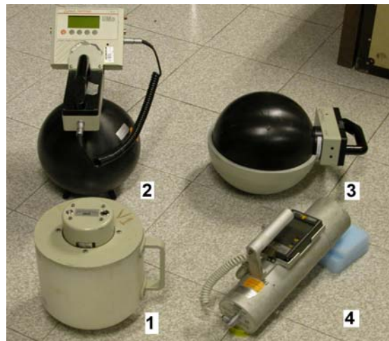
Figure 8.11: The monitor instrument (1) and the complementary devices used in the spectrometric / dosimetric measurements around the DAΦNE accelerator complex. The lead loaded LB6411-Pb (n. 3) is presented with only half lead shielding. The AUTOMESS 6150 AD-b (n.4) has been used to estimate the photon dose.
