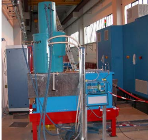
Figure 1.2: A modern klystron with its power supply at the LNF. Even though the manufacturer shielded a large part of the device, yet additional lead foils were necessary to protect the surrounding working area.
