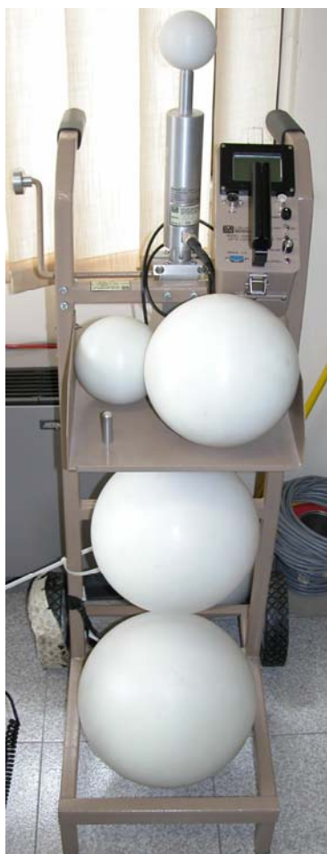
Figure 3.4: The mobile unit used to transport the spheres and perform the irradiations in reproducible geometry.
