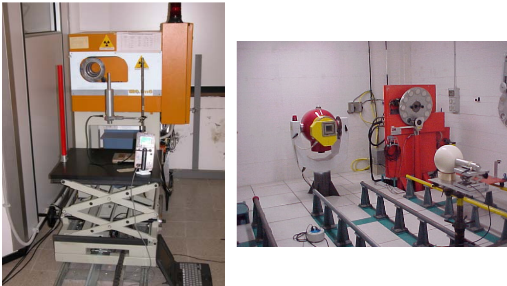
Figure 3.5: The LNF spectrometer being exposed in the gamma irradiation unit of the LNF (left) and ENEA (right) Secondary Standard Calibration Laboratories.
