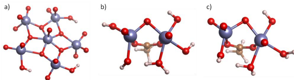
Figure 5.7: CP-MD structures after equilibration run: the three-protonated pentagonal motif (a) and the linker unit (b and c).
