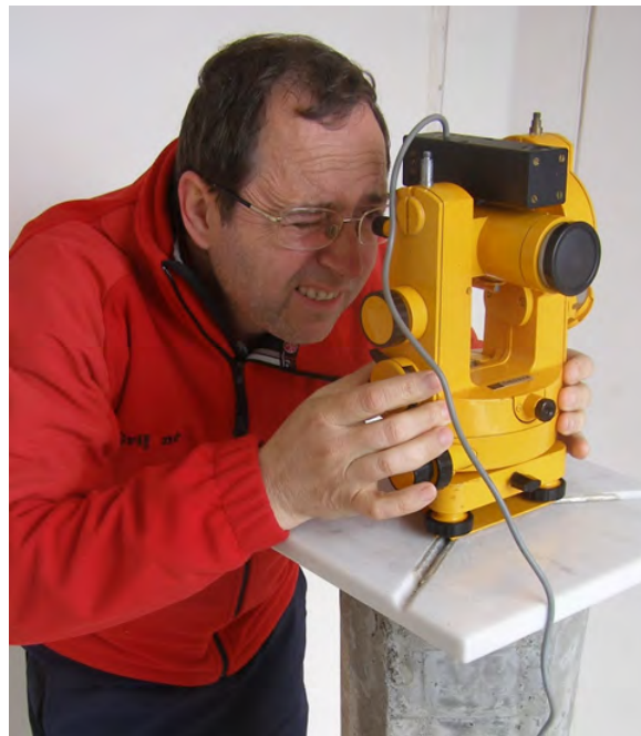
Fig. 6.2 The manual D/I fluxgate theodolite being manipulated by a specialist.
