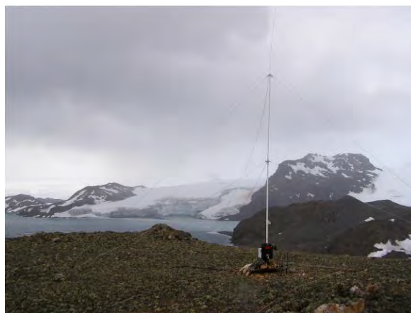
Fig. 6.7 The antenna of the oblique ionosonde transmitter in the ASJI.
