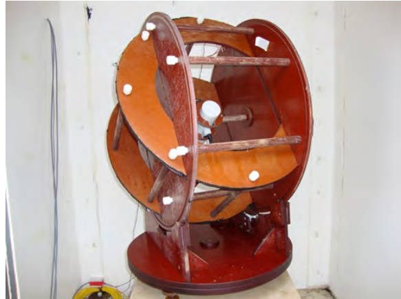
Fig. 6.3 \delta D/\delta I vector magnetometer deployed at the ASJI with the two perpendicular pairs of Helmholtz coils and the Proton magnetometer allowing to measure the variations of D/I.
