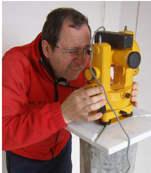
Figure 2. The manual D/I fluxgate theodolite being manipulated by a specialist.
