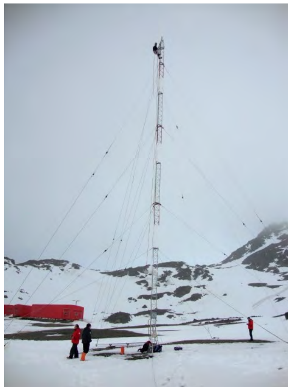
Fig. 6.5 The VIS installed at the ASJI is the Advanced Ionospheric Sounder (AIS) developed by the Istituto Nazionale di Geofisica e Vulcanologia (INGV) of Rome, Italy. For more details about the ionosonde see [9].
