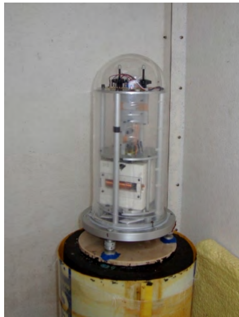
Fig. 6.4 The three-axis automatic fluxgate magnetometer was added in 2008.
