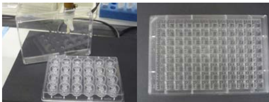
Figure 36. Crystallization plates. Left, a Cryschem 24 well sitting drop plate. Right, a Corning 96 well plate for nanodrops.
