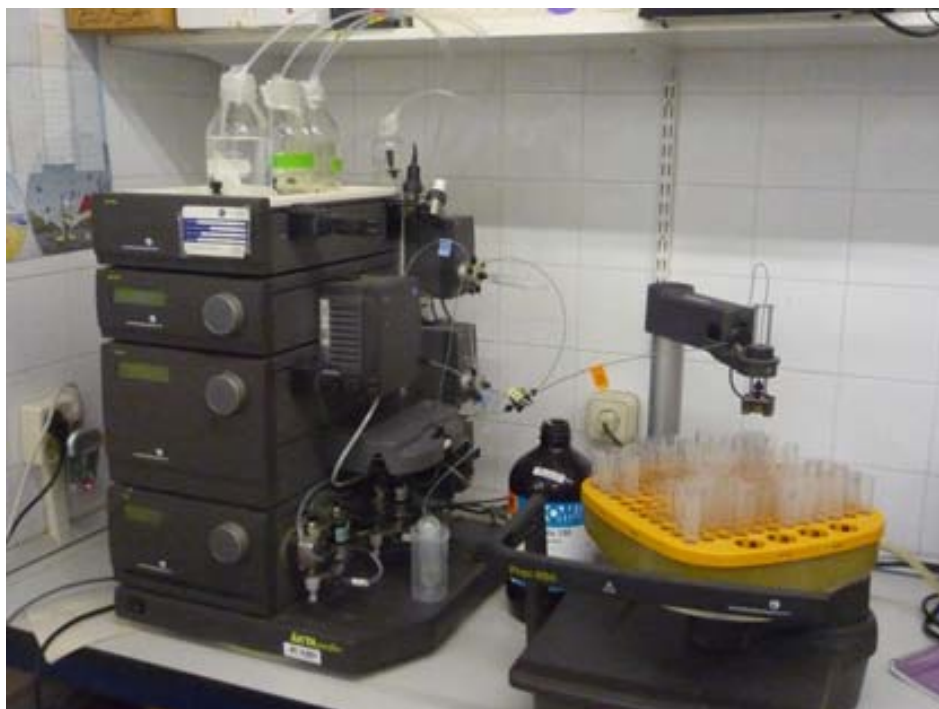
Figure 33. Äkta-FPLC purifier system equipped with fraction collector Frac-950 and external pump P-960.
