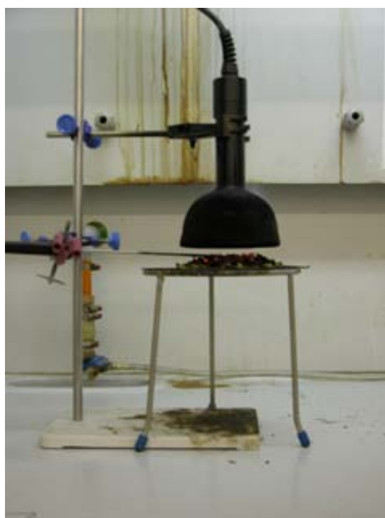
Photograph 1. Picture of the method used to measure flammability. Leaves sample in the smoldering phase under a quartz epiradiator.
