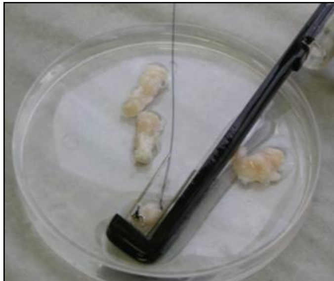
Figure 3. Circular muscle strips disposed on one end and attached to a strain gauge transducer.
