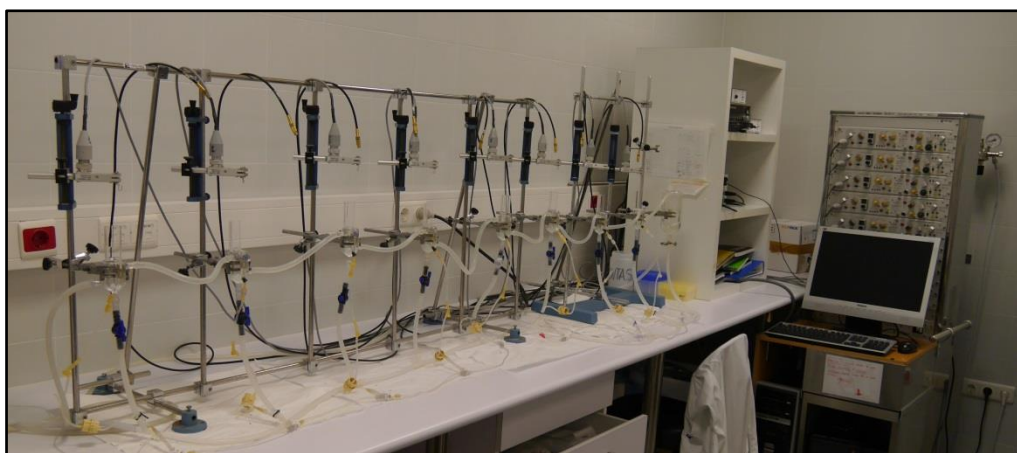
Figure 6. Illustration showing the laboratory with the organ bath chambers, the polygraph and the computer.
