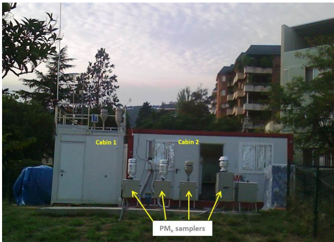
Figure 2.4: UB site monitoring site lay-out. Instruments were located inside two conditioned cabins with their sampling inlets located on the roof. Additionally PM samplers were located outside the cabins.
