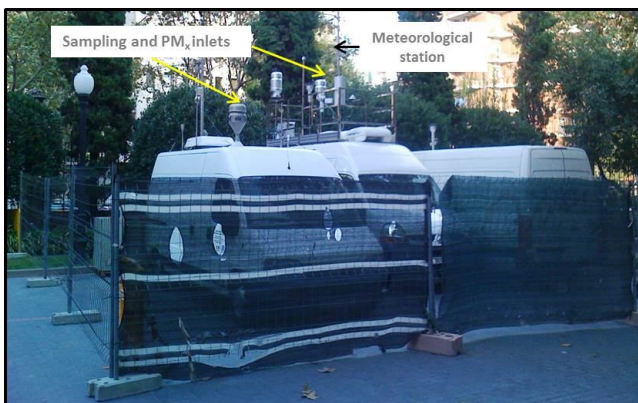
Figure 2.3: RS_{site} monitoring site lay-out. Instruments were located inside the vans with their sampling inlets located on the roof.
