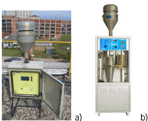
Figure 2.10: High-volume samplers: a) MCV, b) Sequential Digitel.
