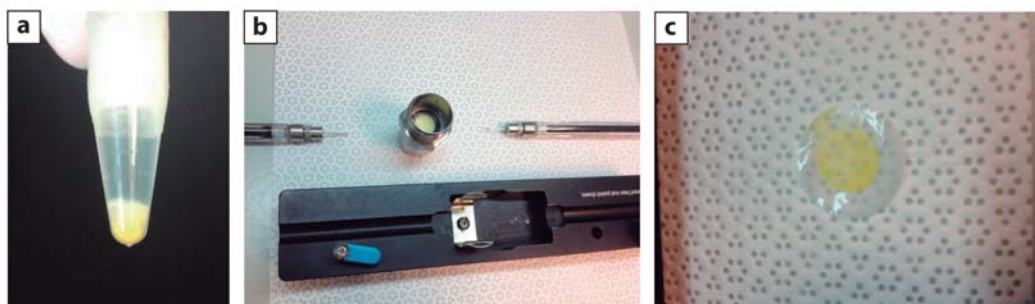
Figure 3.34.: Formation of Chol/Chol-Fc/CTAB aqueous mixture at 0.19 FC ratio by TFH followed by different extrusion protocols. (a) Picture of the sample after the hydration step showing the precipitation of a yellow solid. (b-c) Pictures showing the yellow solid retained in the membrane filters after extrusion process.
