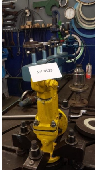
Figure 6-32. Picture of YS3925 ready to do the test (see the bottle with water to count the bubbles).
