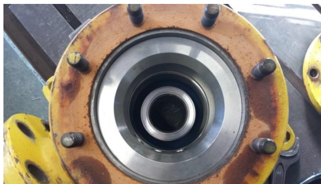
Figure 6-29. Picture of the seating surface of 6510B. It is in good condition after machine and leap.
