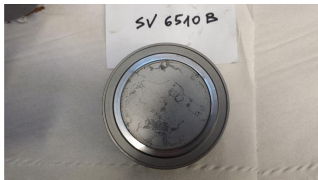
Figure 6-28. Picture of the disc of 6510B. Detail of deposits and corrosion on the disc.
