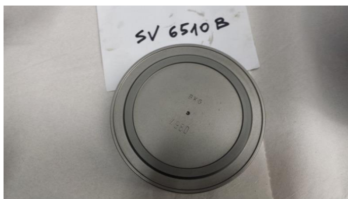
Figure 6-30. Picture of the disc of 6510B after lapping process.
