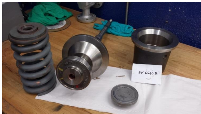
Figure 6-27. Picture of 6510B disassembled (light corrosion on the disc and on the spring can be appreciated).
