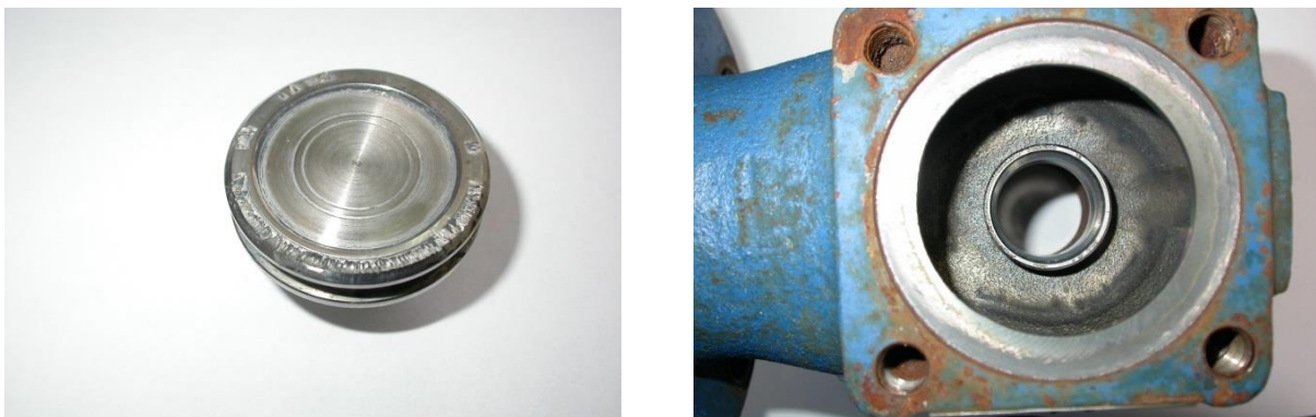
Figure 4-4. Typical damage in the disc and the seating surface of a safety valve because of chattering.
