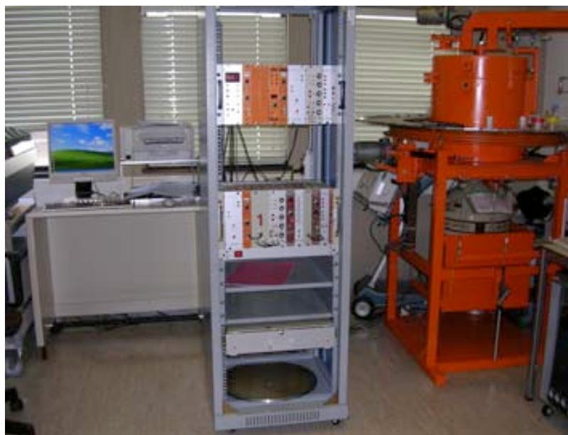
Figure 2. \gamma -spectrometry system with Ge crystal and autosampler.
