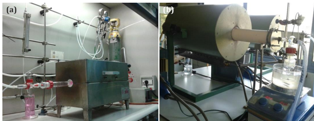
Figure 2.1. (a) Ammonolysis system employed for the preparation of nitrogen-modified materials. (b) Purification system employed for the elimination of amorphous carbon and graphitic particles from CNT samples.
