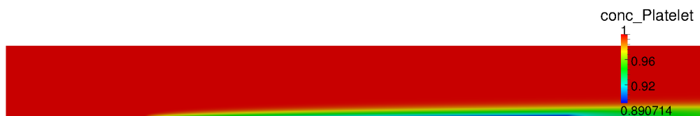
Fig. 5.6 Test case for a Schmidt number of 23, Péclet number of around 446 (based on the shear rate and reacting surface) and a constant reaction rate k_{rt} = 10^{-4}m/s . This is a qualitative image to show the steady mass transport boundary layer thickness.
