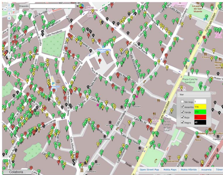
Figure 6-8 Online post-earthquake damage survey database for Lorca
