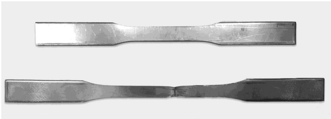
Fig. 3.2. Austenitic stainless steel coupons before and after testing.
