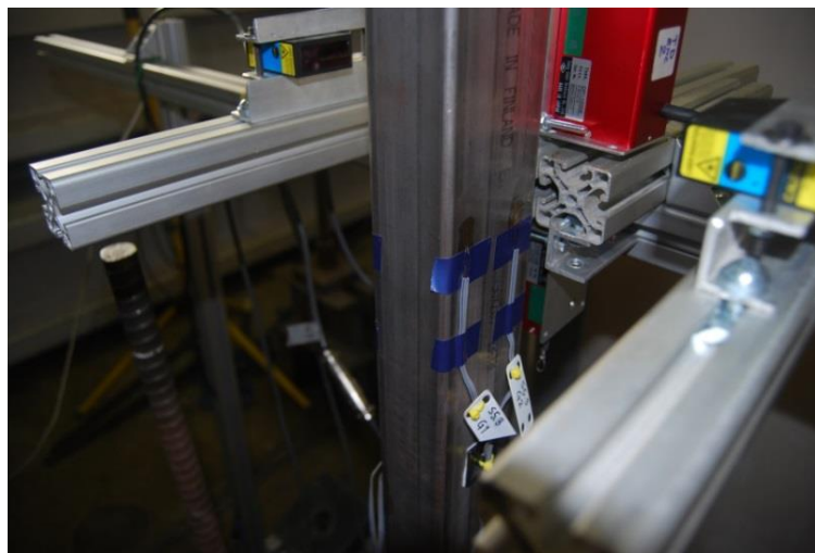
Fig. 4.24. In detail instrumentation setup at mid-height section.
