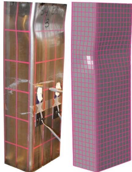
b) Experimental and FE failure modes
