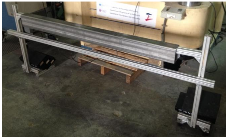
Fig. 4.5. Global geometric imperfection measurement setup.
