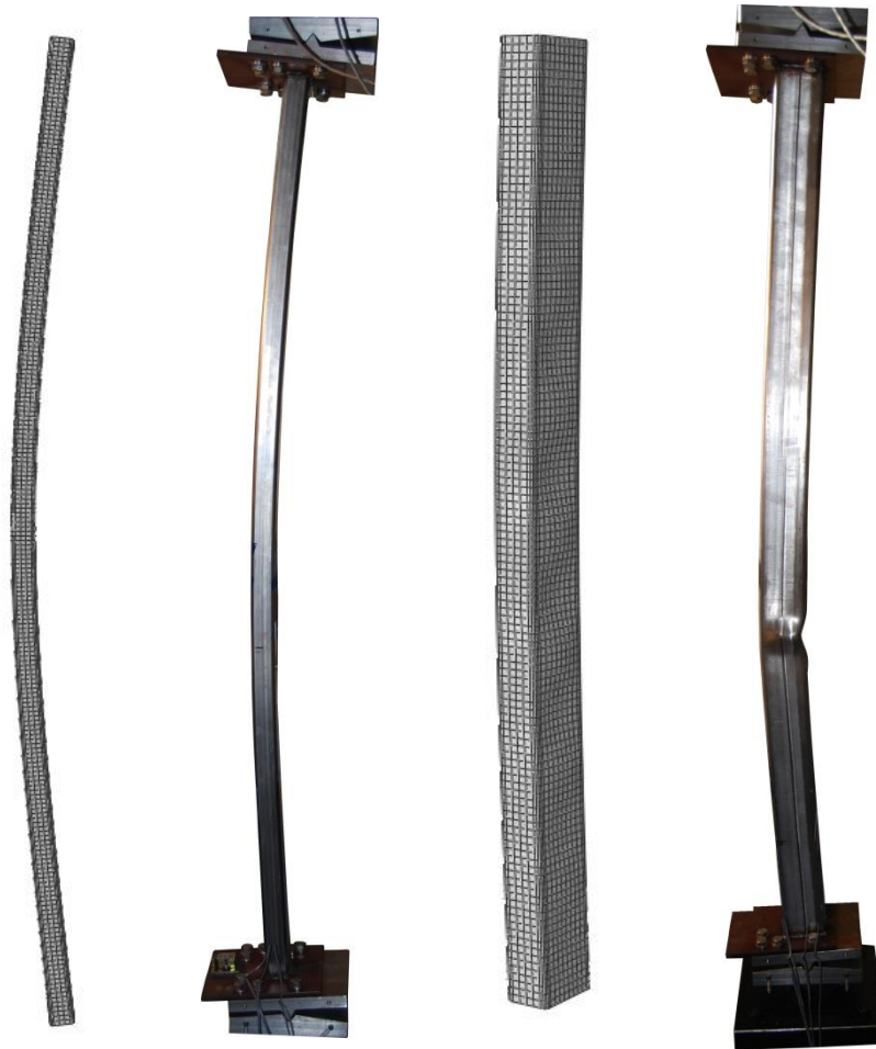
Fig. 5.4. Comparison of the experimental and numerical deformed shapes for S3 and S4 specimens.
