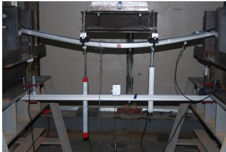
Fig. 4.12. General view of the S3-Mi – 4P test under four-point bending conditions.
