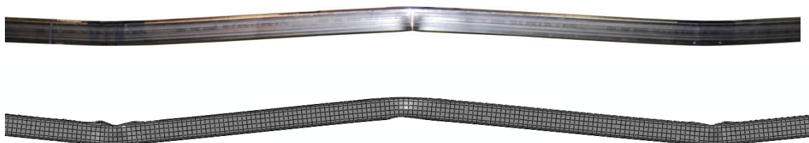
Fig. 5.5. Comparison of experimental and numerical deformed global shapes for a typical continuous beam.
