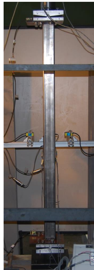
Fig. 4.26. S1 – CC specimen prior to testing.
