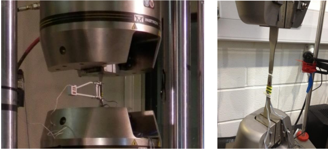
Fig. 3.3. Tensile coupon tests conducted at UPC and Imperial College London.
