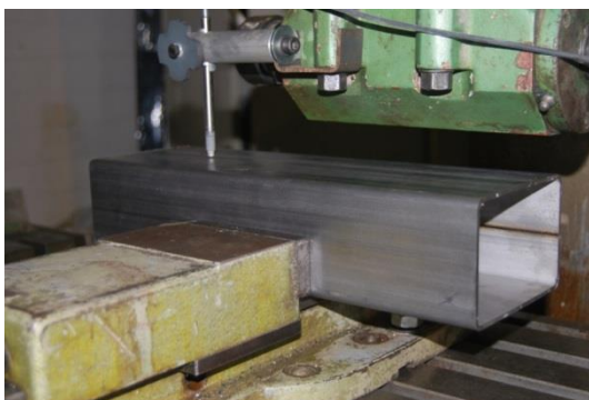
a) Local imperfection measurement setup
