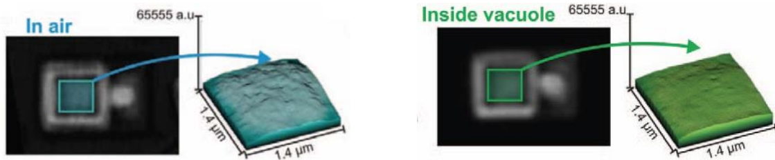
Figure 5.40: CSLM image quality. Representative reflective images (left) and displays of a three dimensional graph of the intensities of pixels framed at centre of the membrane (right) for chips a) in air and b) inside a vacuole.
