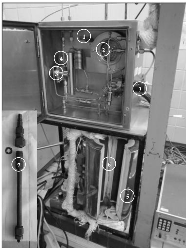
Figure 2.3. Photography of the hot box, electric furnace and reactor (1-hot box thermocouple, 2-hot box heating unit, 3-4-way valve, 4-evaporator thermocouple, 5-tubular furnace, 6-reactor thermocouple, 7-reactor)
