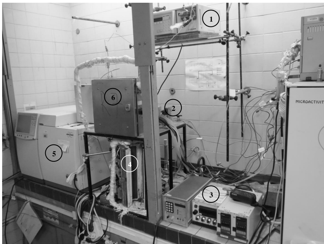
Figure 2.2. General view of the reaction system (1-liquid pump, 2-gas connections, 3-control devices, 4-tubular furnace, 5-gas chromatograph, 6-hot box)
