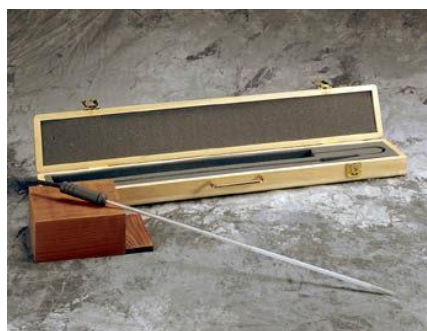
Figure 2.3: Picture of a Standard Platinum Resistance Thermometer (SPRT 25 \Omega ). Image source: INRiM
