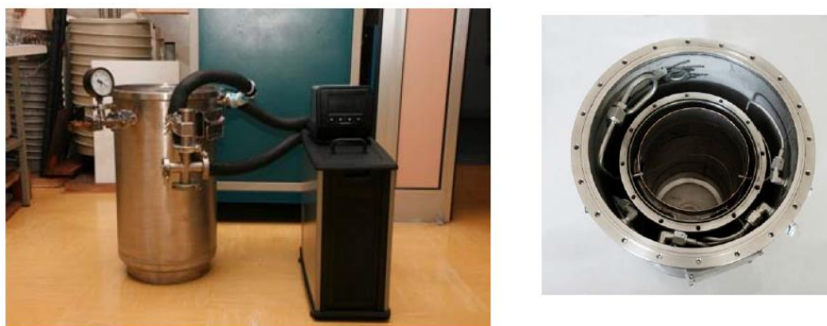
Figure 3.5: The climatic chamber EDIE-1. Image source: MeteoMet project
