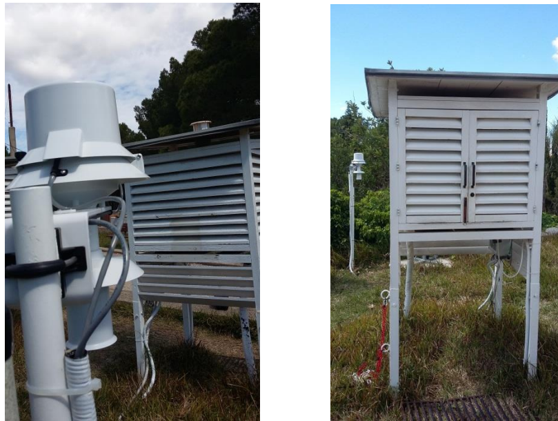
Figure 3.4: Pictures of the new sensor inside a Young – aspirated Screen. Image source: A. Gilibert
