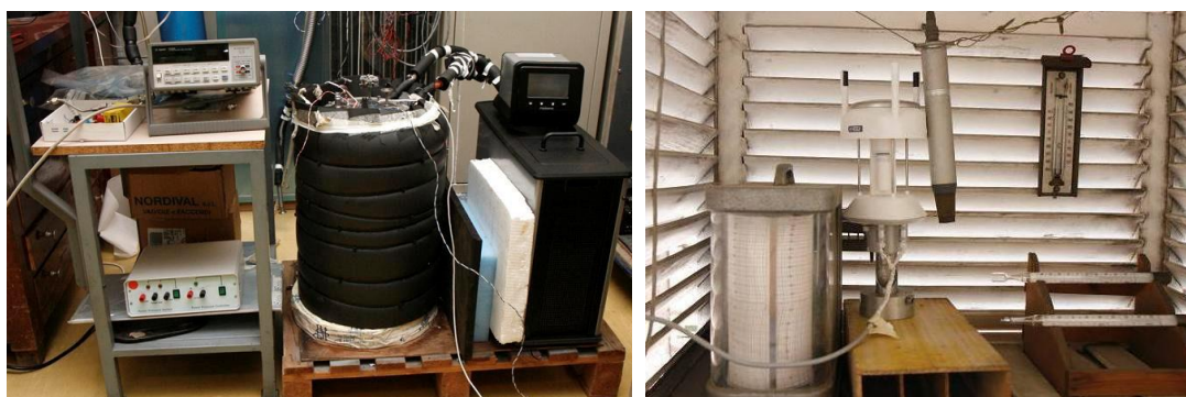
Figure 3.7: Picture of EDIE-0 and the interior of the Stevenson Screen. Image source: MeteoMet
