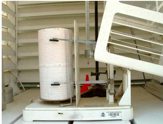
Figure 2.8: A thermohygrograph. We can see the arm and the pen, the band and the drum that rotates driven by a clockwork system. Source image: Ebro Observatory
