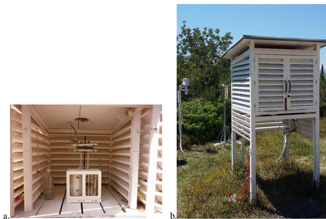
Figure A1.7: Image inside the Stevenson Screen (in which there is installed the AWSc 1) and image of the Stevenson Screen and at rear the Young Screen (in which there is installed the AWSc 2). Image source: A. Gilabert
