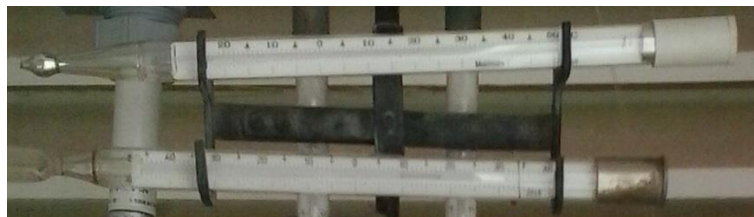
Figure 2.7: Fuess maximum and minimum liquid-in-glass thermometers, installed in Ebro Observatory. Source image: A.Gilabert
