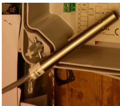
Figure 2.4: Platinum Resistance Thermometer (Pt100). Pt100 installed in Ebro Observatory field trial. Source image: A. Gilibert
