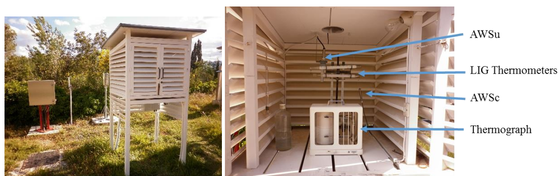
Figure 3.3: On the left the image of the Stevenson Screen in which are placed the different temperature instruments. On the right, a view of the interior of the Stevenson Screen: the LIG Thermometers, the AWSu, the AWSc and the thermograph. Image source: A. Gilabert
