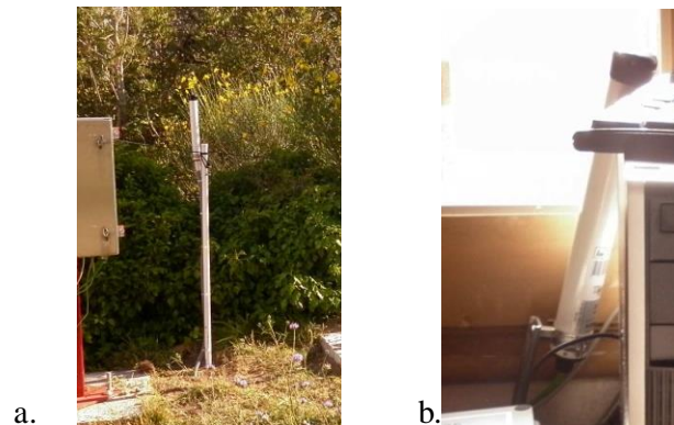
Figure A1.4: Image of the two antennas, (a) connected to the measuring and transmitting module and (b) connected to the receiving module. Image source: A. Gilabert
