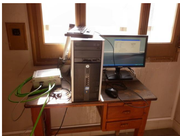
Figure A1.6: The computer that stores the data and in which is installed the program which manages the temperature measurement system and transforms the data. Image source: A. Gilabert
