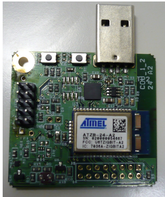
Figure 3.3: A COU24-A2 development board. The COU24-A2 board features an Atmel ATmega-1281 microcontroller and an Atmel AT86RF20 transceiver.
