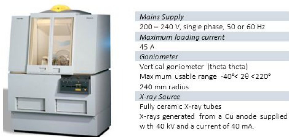
Figure 2.10. Image and specifications of XRD instrument.
