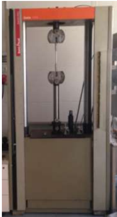
Figure 3.10. Vertical bench of 5 tons used to perform the mechanical tensile tests.
