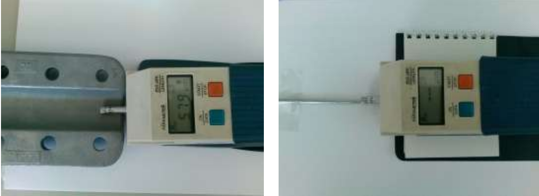
Figure 4.16. Roughness measurements performed with Mitutoyo Surftest 211 surface roughness tester on both connector's and conductor's surfaces.
