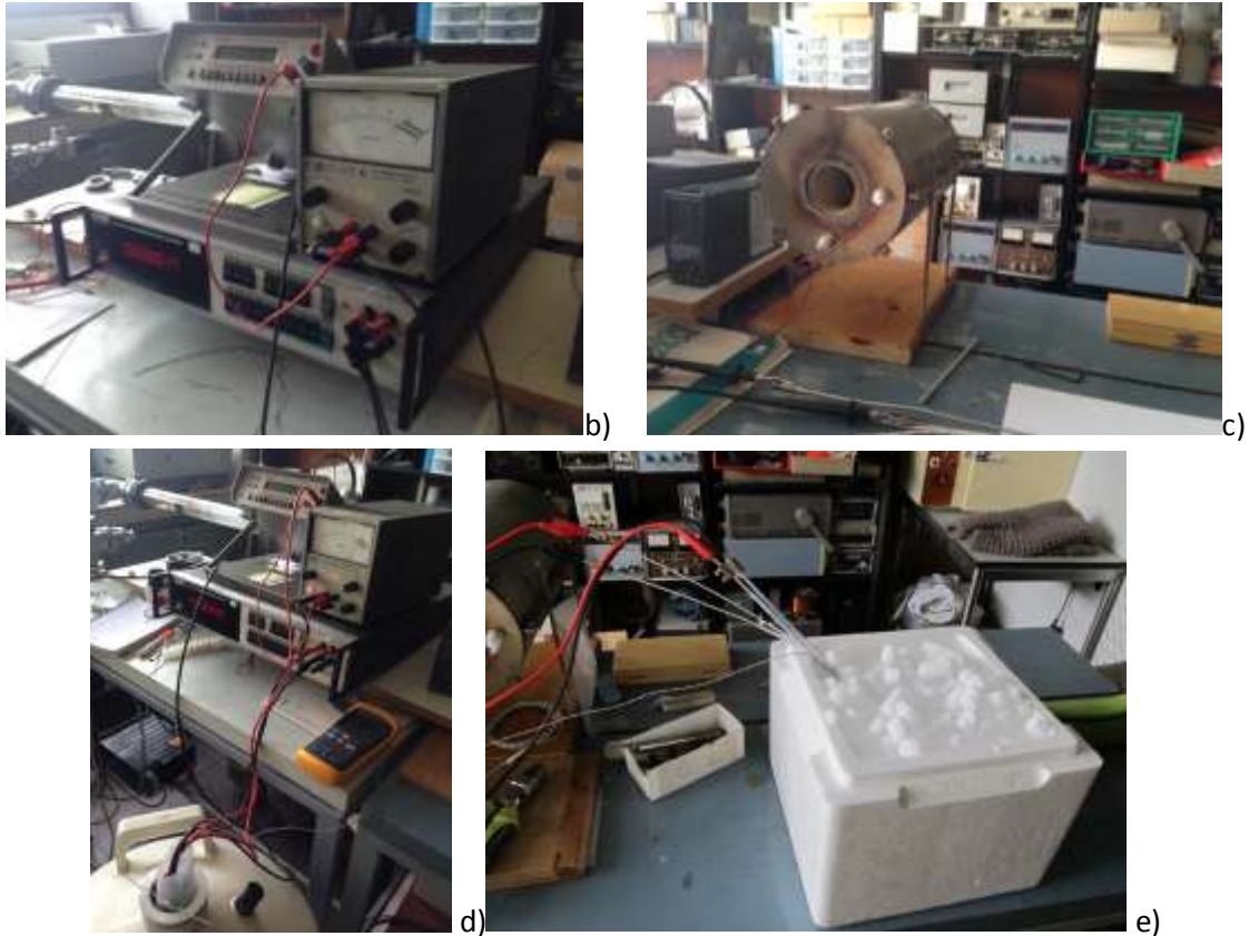
Figure 3.12. Experimental setup for the measurement of the temperature coefficient of electrical resistivity a) Simplified scheme of the test setup for the measurement from room temperature to 200^{\circ}\text{C} . b) Stabilized current source and voltage and current measurement system. c) Temperature-controlled electric oven d) Resistance measurement of the test specimen at temperature of boiling point of liquid nitrogen stored in a vacuum flask. e) Resistance measurement of the test specimen at temperature of sublimation temperature of dry ice placed in an insulated box .
