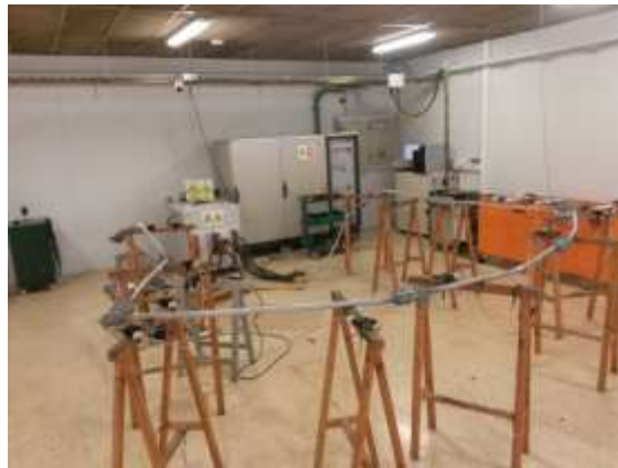
Figure 4.8. Heat-cycle test. Experimental setup.
