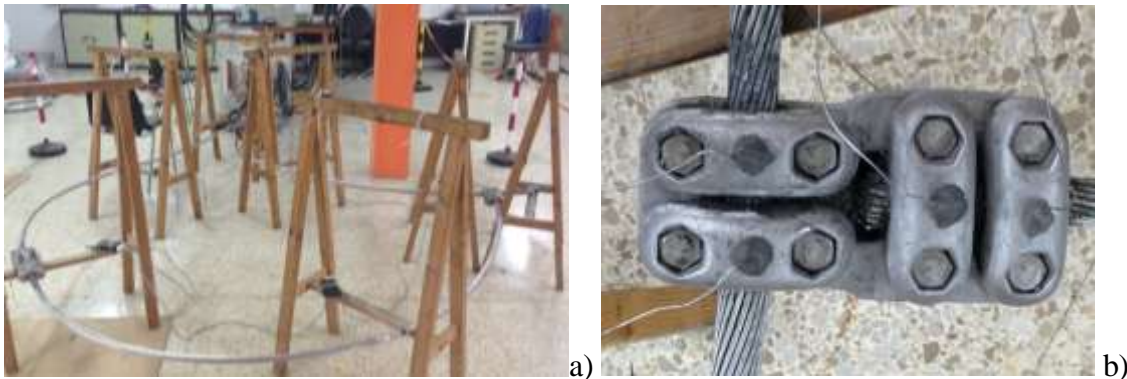
Figure 5.17. Experimental test setup. a) Test loop composed of an ACSS conductor, a T-connector S210ZTLS and two terminal connectors S210ZA4P23LS. b) T-connector S210ZTLS. The five thermocouples placed in the different parts of the connector.
