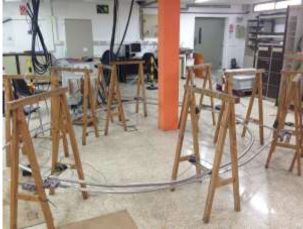
Figure 0.10. Experimental test setup. Outer loop composed of an ACSS conductor, a T-connector S210ZTLS and four terminals S210ZA4P23LS. The internal loop is made of an aluminum stranded conductor with diameter of 32 mm.
