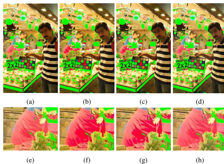
Figure 6.10: Example of artifacts. (a) Ground Truth. (b) Output of CE algorithm [Laird et al., 2009]. (c) Output of LCA algorithm [Laird et al., 2009]. (d) Output of our GEA-LAB2. (e)-(h) Zoomed-in view of the regions cropped from the top row. Note that these are wide-gamut images where out-of-sRGB pixels are masked green.
