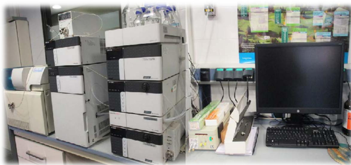
Fig. 3.8 Image of the liquid chromatography-mass spectrometry (Shimadzu LCMS-2010)
