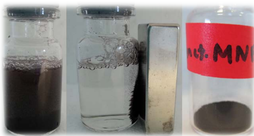
Fig. 3.10 Magnetic nanoparticles separated using a magnetic drive and final product after dried
