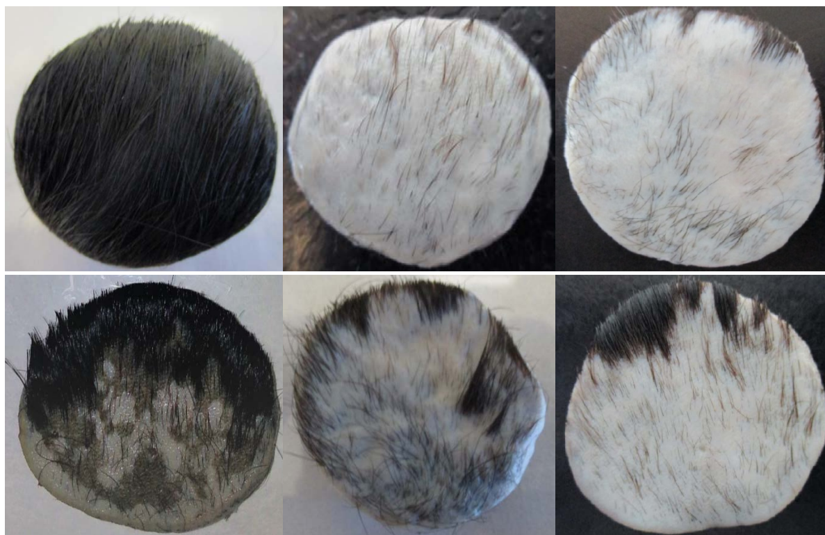
Fig. 4.9 Dehairing of cow hides treated with (a) Tris buffer as control; (b) chemical dehairing; (c) commercial enzyme; (d) protease from R1; (e) protease from R2; (f) protease from R3.
