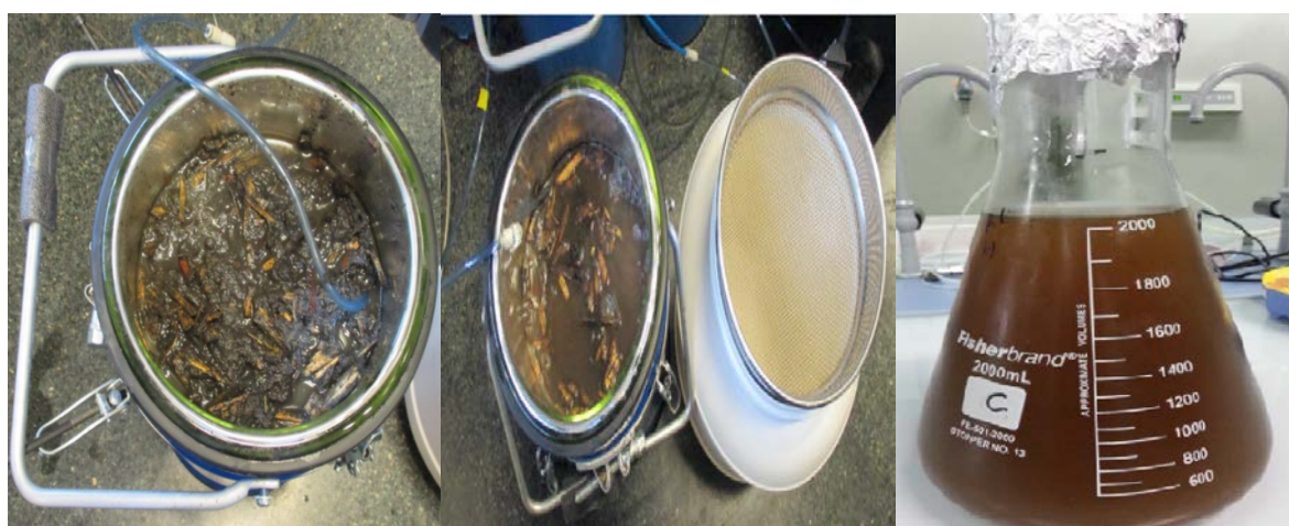
Fig. 3.6 Extraction of whole fermented materials in a single reactor, (a) air bubble supplied to extract the bioproduct from the solid substrate; (b) stainless steel mesh used to separate the solid and liquid extract; (c) image of crude protease extract.
