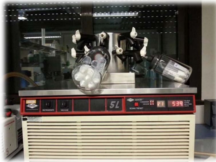
Fig. 3.7 Lyophilisation using a vacuum bench top VirTis Sentry 5 L freezes dryer.
