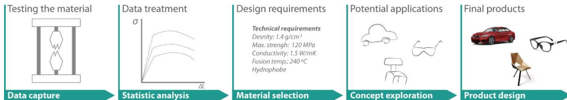
Figure 1.8. Steps to move new materials into successful products Source: Adaptation from (Ashby and Johnson, 2002)
