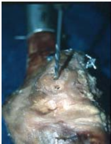
Figure 1: Image For 6 Holes To Pass The Strain Gauges Through Its.
