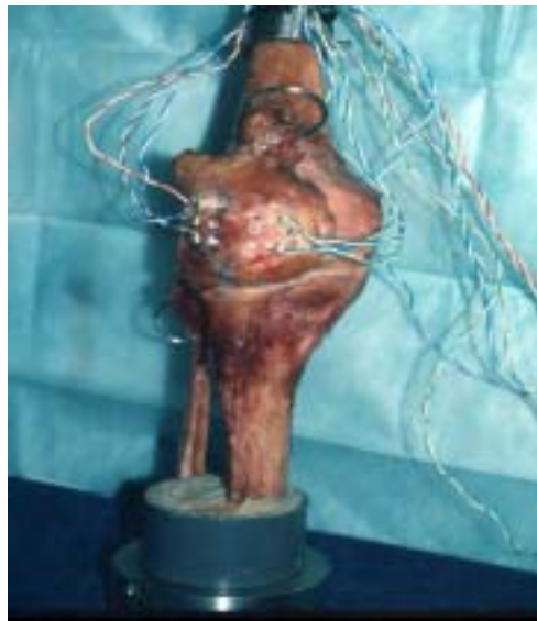
Figure 4: Anterior View Of The Knee With One Ring Attached With Quadriceps Tendon And Another Ring Attached With Femoral Biceps Tendon.
