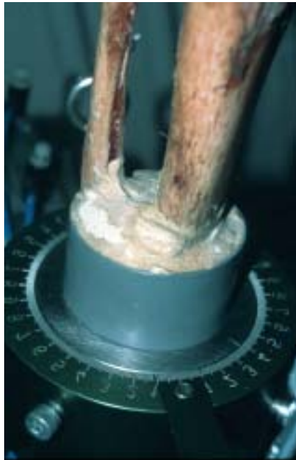
Figure 12 : ( Above Picture Shows That We have used to control the degrees it is the assembly of the system of inclusion on the distal platform that also of anteversion )
