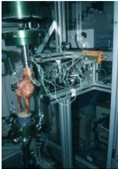
Figure 7: The Specimen Fixed To The Special Device And Was Clamped Rigidly Into Steel Cylinders.
