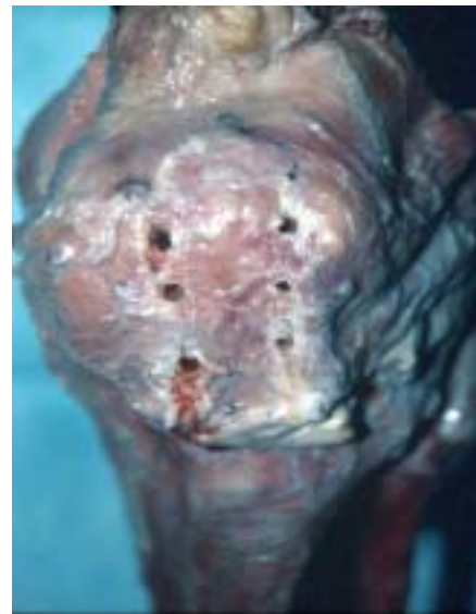
Figure 1: Image For 6 Holes To Pass The Strain Gauges Through Its.
