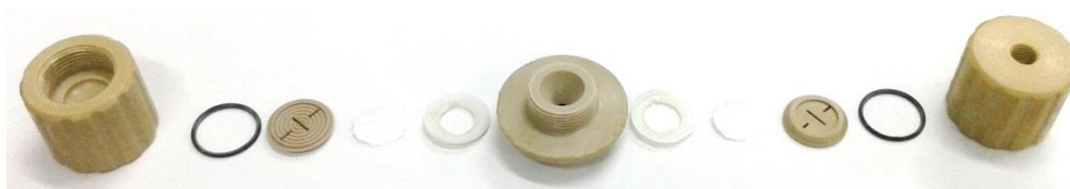
Figure 1.10. Packed microcolumn showing the outer caps, airtight o-rings, filter support, Nylon membrane and washer and low-volume central biconical body.
