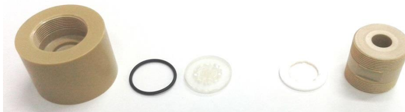
Figure 1.9. Disassembled packed macrocolumn showing (left to right) the outer cap, o-rings for air proofing, a support for the commercial filter, polytetrafluoroethylene (PTFE) washer and central body.
