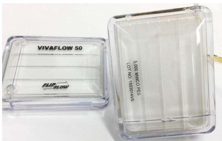
Figure 1.8. Diafiltration cassette used in chapter 10 with details of input/output connections, composition and molecular weight cutoff (MWCO)
