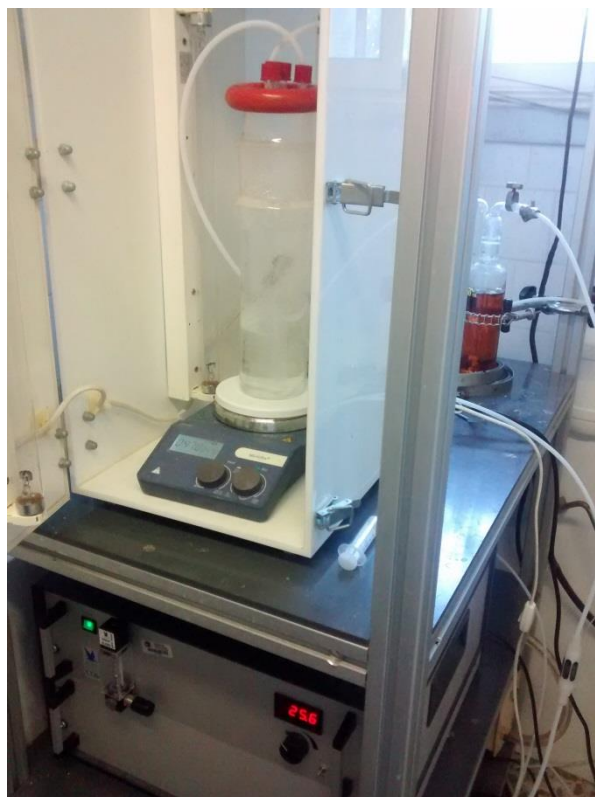
Figure 4.8. Ozone generator and equipment for ozonation experiments
