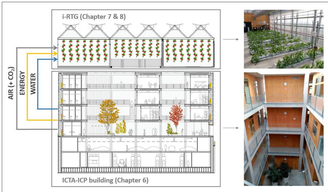
Figure 2.8 Conceptual diagram of the connection between the i-RTG and the ICTA-ICP building.
