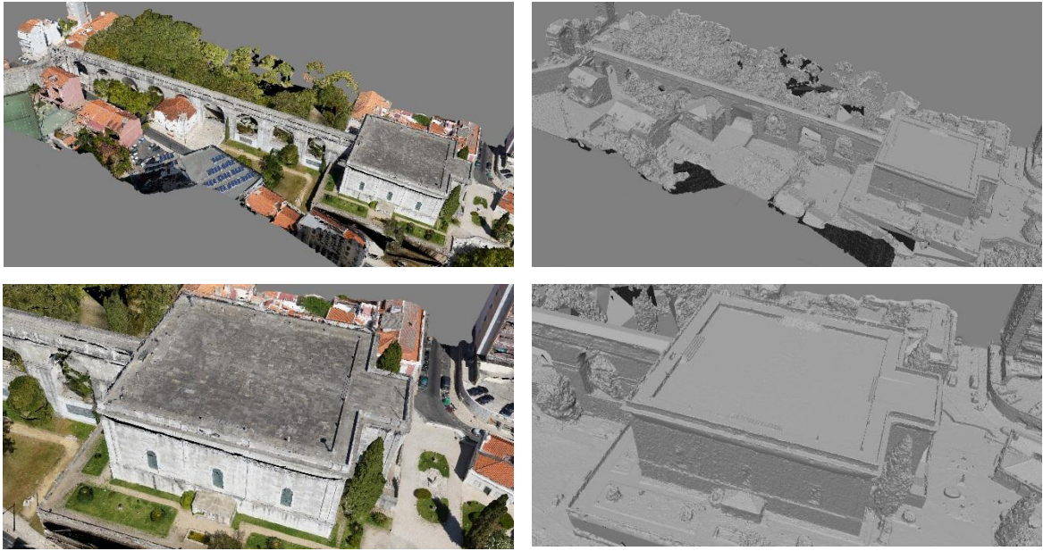
Fig. 60 – 3D modelling of the Mãe de Água (Lisbon Aqueduct System) and detailed area results using Agisoft Photoscan software. Source: images by GEODRONE, 12-03-2016.
