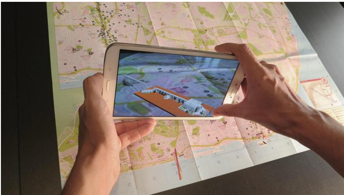
Fig. 69 – Mãe de Água reservoir 3D model and AR environments using the city map as a marker.
